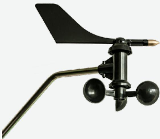
WDL-1 uses a three cup anemometer for high accuracy, sensitivity and durability. The cups are connected to a shaft which turns a sensing element that converts the rotation into a series of electronic pulses.
