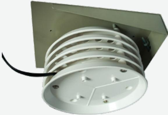
Both Temperature and Humidity are built into the Radiation shield at the bottom of the assembly. The integral shield limits errors due to solar radiation. The RH sensor is a capacitive element enclosed in a protective membrane.
